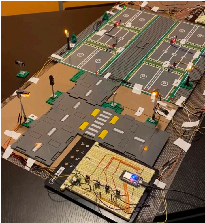
The UF Smart Campus model, featuring LED street lights and sensors for parking spots.
